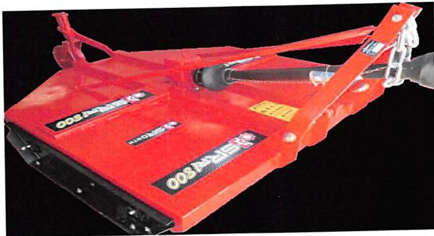
SRR 1800 ROÇADEIRA 1.80 METROS DE CORTE, GIRO LIVRE, EMBREAGEM, 2 FACAS, RODA, CAIXA A ÓLEO, PESO 425 KG, COMPRIMENTO DE 2400 MM, LARGURA 2000 MM, ALTURA 900MM, POTENCIA REQ. 50 CV.
